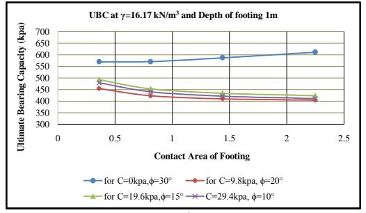
Figure 4: UBC at  $\gamma$ =16.17 kN/m<sup>3</sup> and Depth of footing 1m
