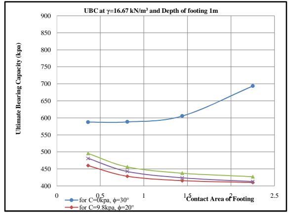
Figure 6: UBC at  $\gamma$ =16.67 kN/m<sup>3</sup> and Depth of footing 1 m
