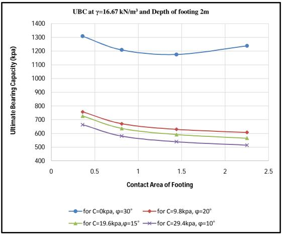
Figure 7: UBC at  $\gamma$ =16.67 kN/m<sup>3</sup> and Depth of footing 2 m
