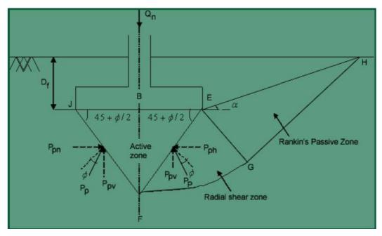
Figure 1: Failure zone considered by Meyerhof
