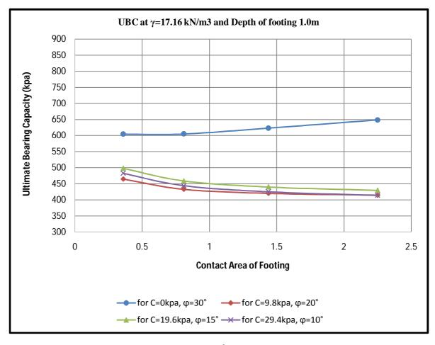
Figure 8: UBC at  $\gamma$ =17.16 kN/m<sup>3</sup> and Depth of footing 1 m
